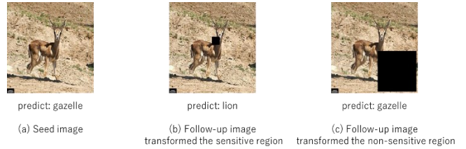
Fig. 1. Example of MT that add a black dot. A seed image classified as a gazelle (a). A follow-up image added a black dot inside the sensitive region (b). A follow-up image added a black dot outside the sensitive region(c).
